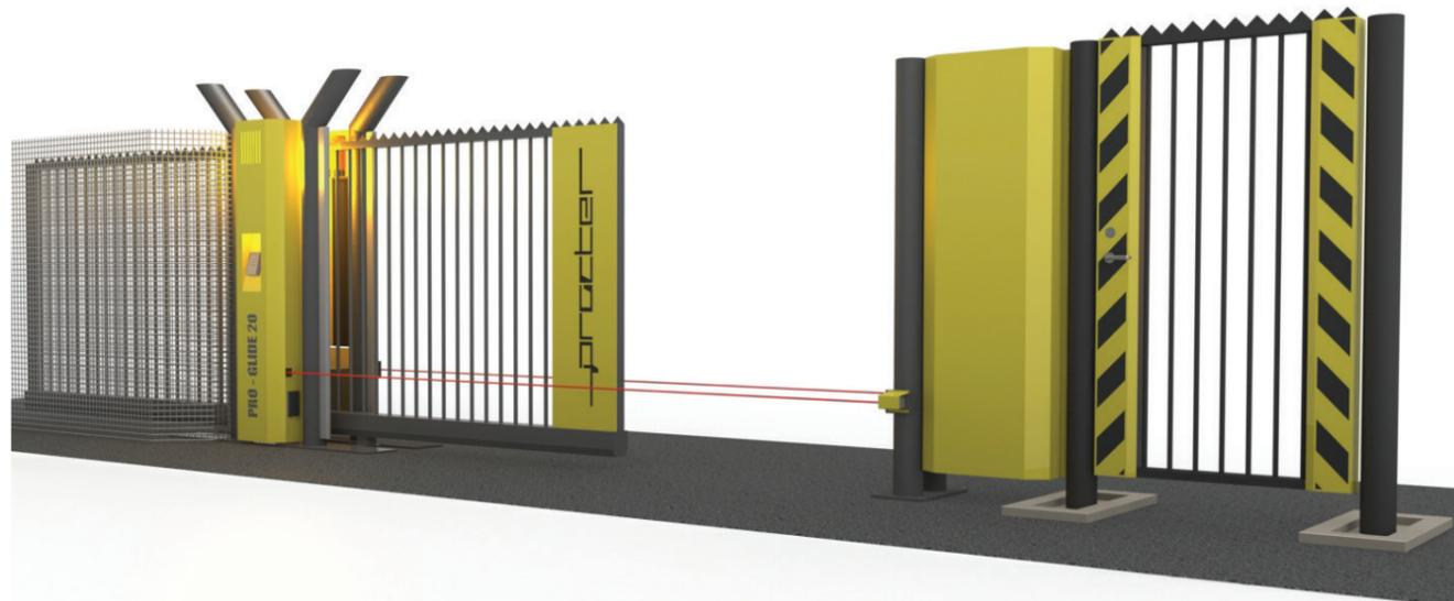
There are advantages with both cantilevered and tracked, and it's really a case of which is most appropriate to an individual site. There are a number of considerations but in essence cantilevered gates have the advantage of being able to run over an uneven surface (because the gate is above the ground), with tracked gates being more suitable for very wide openings. In any event when required to do so, we will always advise on the best option.
